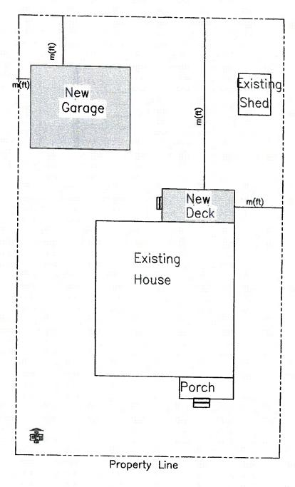
A site plan identifies buildings and other features in relation to property boundaries. The site plan should identify your existing Structures (ie. house, garage, deck, shed etc) and your proposed addition or new structure
